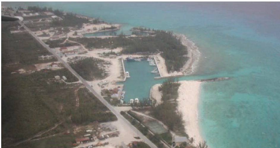
Figure 20. The groyne-protected entry to this marina on San Salvador has caused the loss of the entire sandy beach to the south (top of picture), but widened the beach in the north. Long-shore drift on the SW coast of San Salvador is from north to south in this location. Credit: Neil Sealey.
